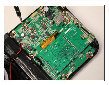
Remove (10) screws (7 mm) with a PH1 screwdriver on the motherboard.
