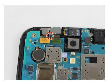
Remove the one 2.55 mm Phillips #000 screw from top left of motherboard assembly.
