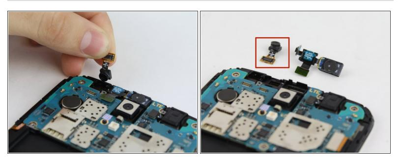
Lift the motherboard connector and remove the camera assembly from phone.
