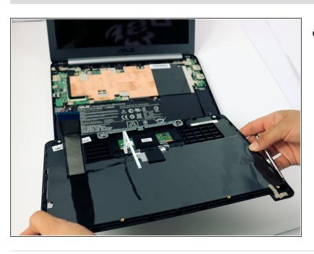
Remove the keyboard cover and safely place it somewhere face down.
