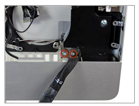
Remove the two 5 mm T10 Torx screws securing the audio ports to the outer case.
