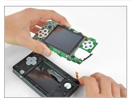
Remove the motherboard assembly from the rest of the device. To reassemble your device, follow these instructions in reverse order.
