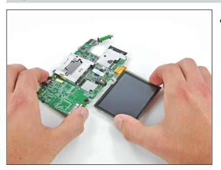
Grasp the lower display assembly and pull it directly away from the motherboard.
