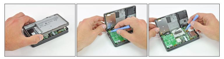
• Lift the bottom edge of the lower case off the rest of the 3DS.
