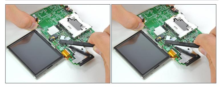
• Use the flat end of a spudger or your fingernail to flip up the retaining flap on the touchscreen ribbon cable ZIF socket.
