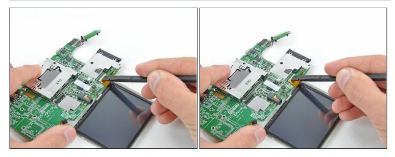
Use the flat end of a spudger or your fingernail to flip up the retaining flap on the lower LCD data ribbon cable ZIF socket.
