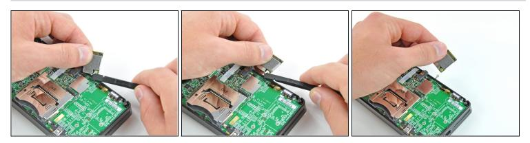
(i) Lift the Wi-Fi board off the motherboard and rotate it so that the bottom side is facing up.
