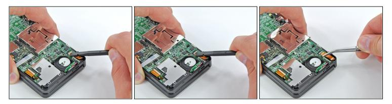
Use the flat end of a spudger or your fingernail to flip up the retaining flap on the speaker assembly ribbon cable ZIF socket.
