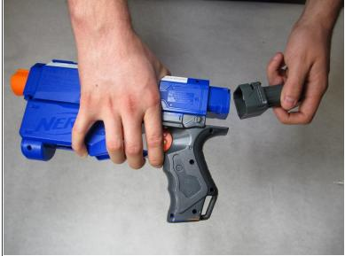
Remove the stock attachment point by removing the two 8mm Phillips head screws.
