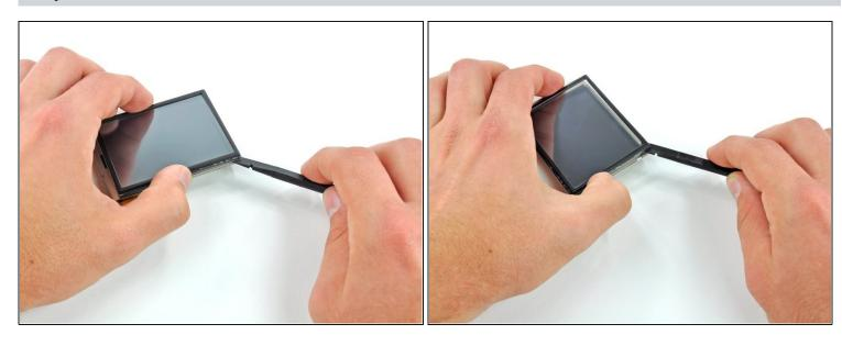
Repeat the above procedure for the remaining two corners to pry the touchscreen off the LCD frame.
