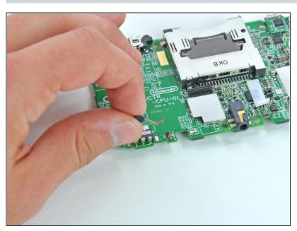
Lift the microphone and its attached ribbon cable off the motherboard.
