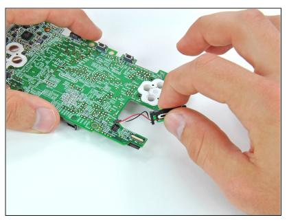
Remove the volume switch from the motherboard.
