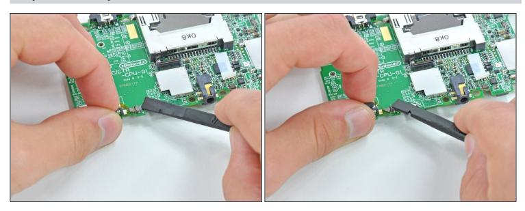
Use the flat end of a spudger or your fingernail to flip up the retaining flap on the microphone ribbon cable ZIF socket.
