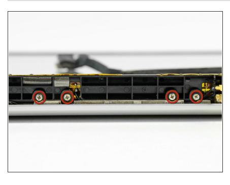
Remove the four 3 mm Phillips screws securing the antenna bracket to the display.
