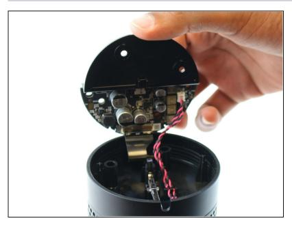
Slowly lift the plate containing the board. Be careful not to disconnect any of the wires.
