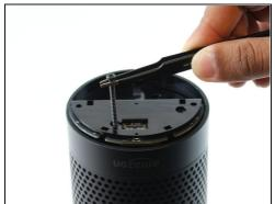
• Remove the four 42.8 mm T10 Torx screws from the bottom of the Echo.
