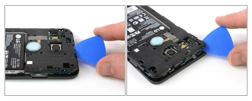
• Continue sliding the opening pick around the upper part of the midframe to release the plastic clips.
