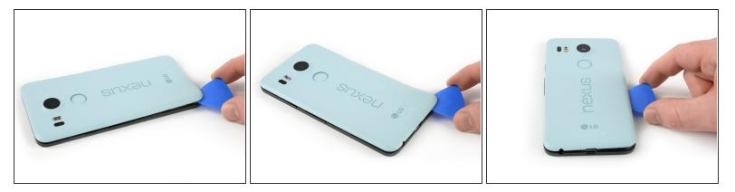
Continue to slide the opening pick around all sides of the phone to release all clips that secure the rear panel.
