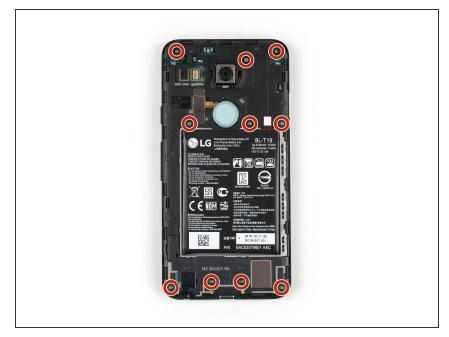
• Remove the ten 3.6 mm Phillips screws that secure the midframe.
