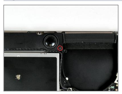
Remove the single Phillips screw securing the subwoofer to the upper case.
