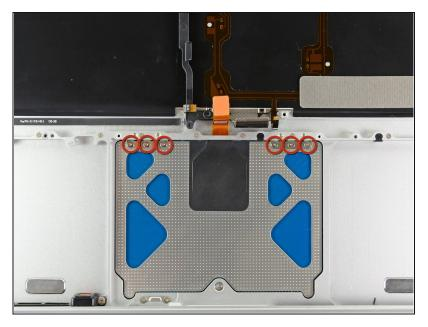
Remove the six 1.4 mm Y0 Triwing screws securing the trackpad to the upper case.
