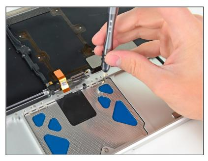
Insert a 1.4 mm Y0 Tri-wing screw into each of the outer holes drilled into the trackpad (two screws total).
