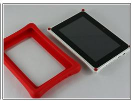
Remove the rubber bumper from the tablet.
