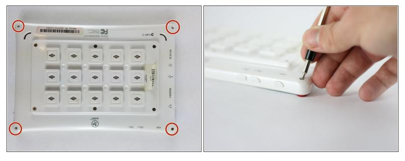
• With a PH00 screwdriver, remove the four outermost screws from the back of the tablet.
