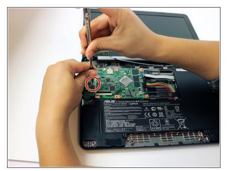
Use a J0 Phillips screwdriver to remove the single, silver, 4mm screw on the motherboard.
