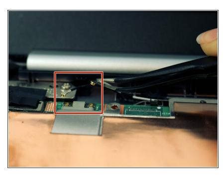
Use the tweezers to disconnect both wifi antenna cables from the motherboard.
