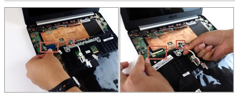
Carefully pull the keyboard cables out of the connecting ports that are attached to the motherboard.
