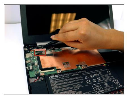
Use tweezers to disconnect the LCD cable from the motherboard.
