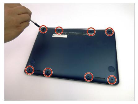
Use the J0 screwdriver to remove the eight 5mm black screws on the bottom of the laptop, which includes the two that were hidden under the rear rubber feet.
