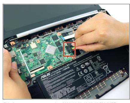
Use the tweezers to disconnect the battery cable from the motherboard.
