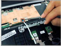
Use the metal spudger to gently pry up the small tabs that are clamping down on the keyboard cables.
