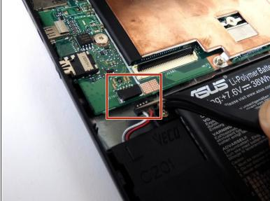
Remove the sound cable from motherboard.
