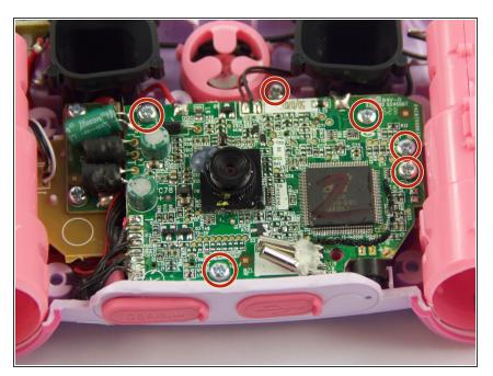
Locate and remove the screws circled in the provided image with a Philips #0 screwdriver.
