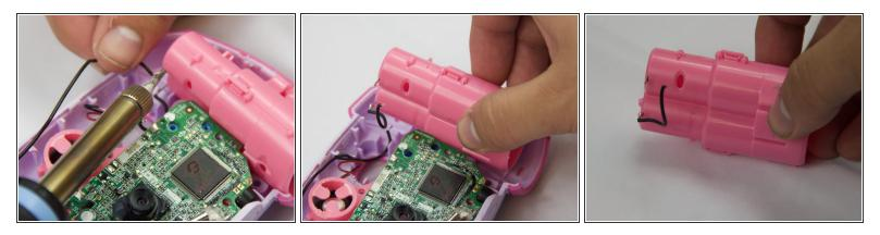
Unsolder the connections to the right battery terminal. Removing the terminal allows easier access to the motherboard.
