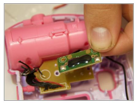
Gently pull up on power distribution circuit board and remove it from the device.
