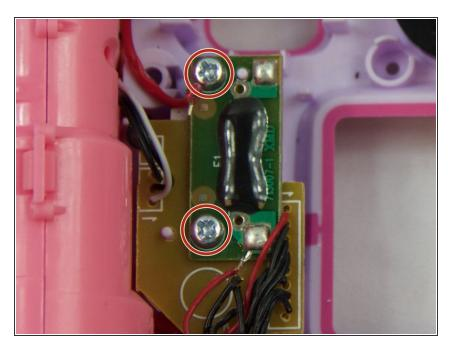
• Locate and remove the two screws that hold in the power distribution circuit board using a Philips #0 screwdriver.
