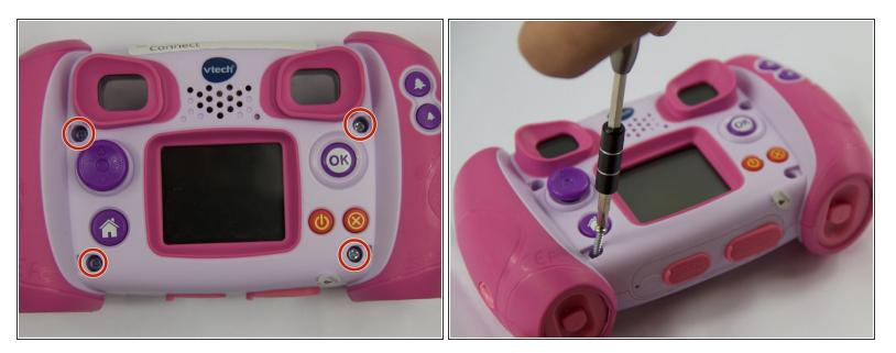
Remove all four (11mm) screws with the Philips #0 screwdriver.
