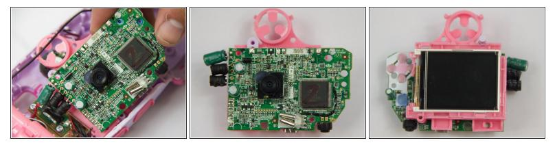
• Carefully pull up on the motherboard and pink plastic underneath the motherboard. The pink plastic contains the display and is connected to the motherboard.
