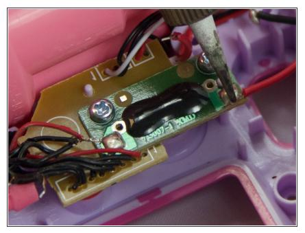
• Unsolder the wires connected to the power distribution circuit board.
