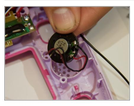
Once the seal is broken the speaker should move freely. Carefully lift and remove the speaker along with its attached red and black wires.
