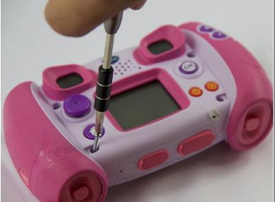
Remove all four (11mm) screws with the Philips #0 screwdriver.
