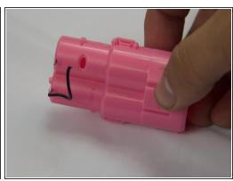
Unsolder the connections to the right battery terminal. Removing the terminal allows easier access to the motherboard.
