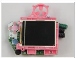
Carefully pull up on the motherboard and pink plastic underneath the motherboard. The pink plastic contains the display and is connected to the motherboard.
