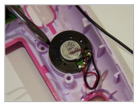
The speaker is glued in so you must use the metal spudger to break the seal made by the glue.
