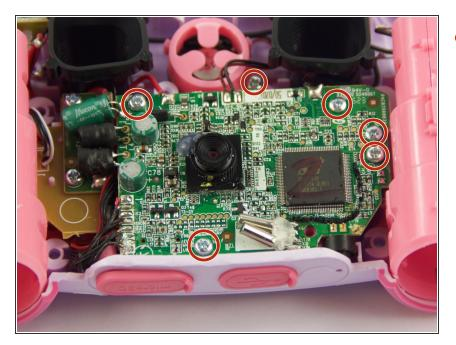
Locate and remove the screws circled in the provided image with a Philips #0 screwdriver.
