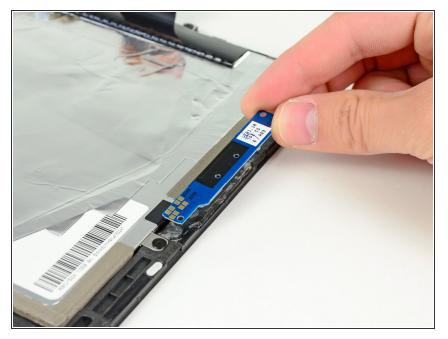
• Remove the home button board from the front panel.
