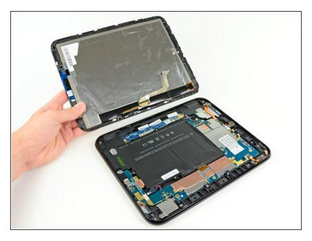
• Remove the front panel assembly from the rear case assembly.
