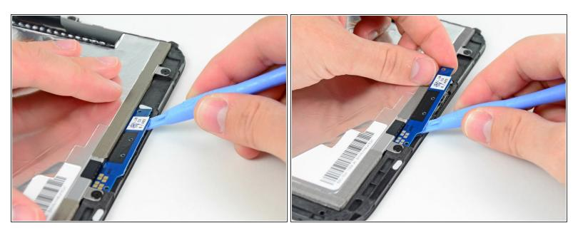
Use a plastic opening tool to pry the home button board off the adhesive securing it to the front panel.
