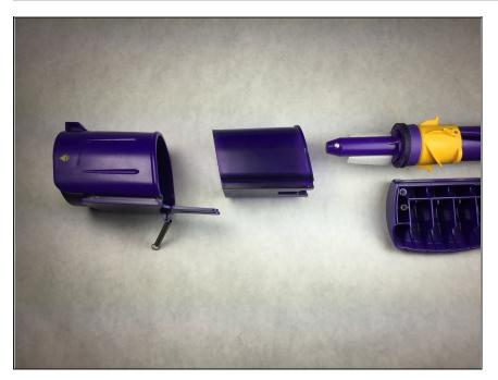
Slide the barrel shield and shield slide off of the gun and set aside.
