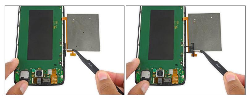
Remove the SIM card holder/volume button rocker.
