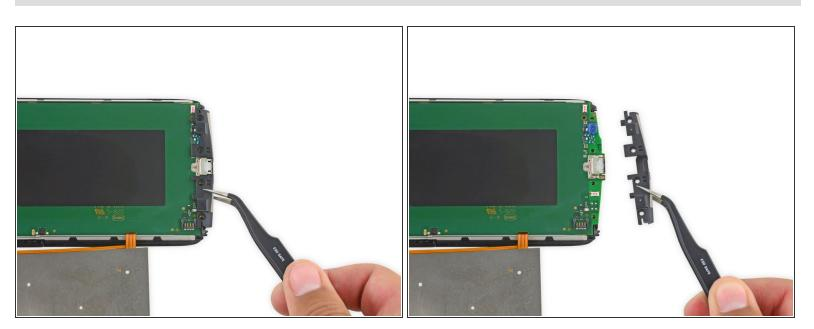
Remove the lower antenna board.
