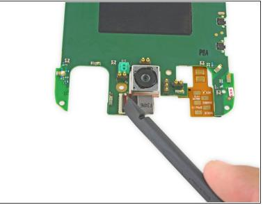
Use the flat end of a spudger to flip up the black retaining flap on the front-facing camera ZIF connector.
