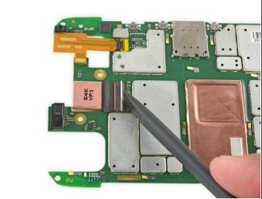
Use the flat end of a spudger to flip up the tan retaining flap on the rear-facing camera ZIF connector.
