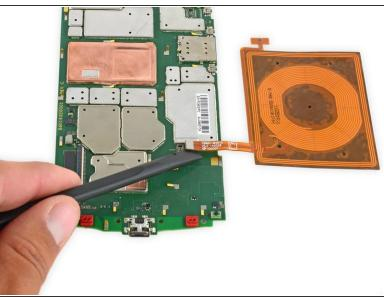
Use the flat end of a spudger to disconnect the wireless charging coil connector from the motherboard.
