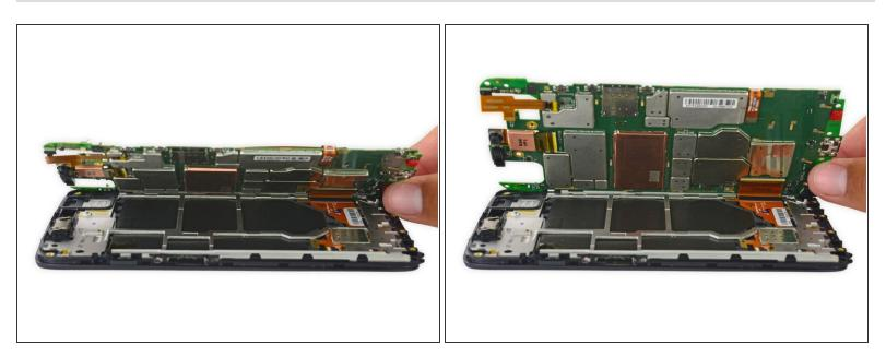
Carefully lift up the motherboard to expose the display connector.
