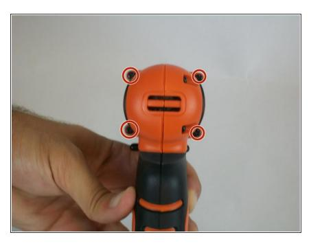
Remove the four screws on the back top side of the drill.
