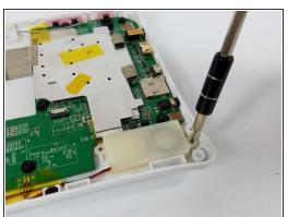
Using a Phillips PH 000 screwdriver, unscrew the two 3 mm Phillips #000 screws on each side of the speakers that hold the speakers in place.
