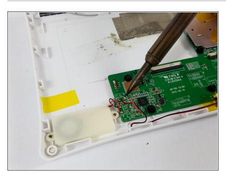
Using the soldering iron, detach the speaker's wires from the circuit board.
