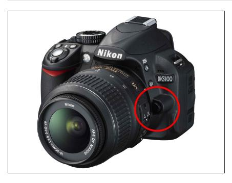
Remove the lens by pressing the release button and twist the lens.
