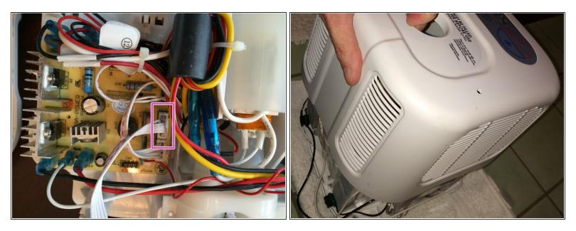
Unhook connector for small ribbon cable which connects control board on top of cube with circuit board on bottom of cube.
