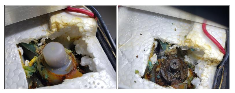
• Added a couple of pictures of the elusive thermal breaker. There are two black wires connected to the thermal breaker. The wires are connected together under normal conditions (closed circuit) and separated (open circuit) when the breaker detects a thermal issue.
