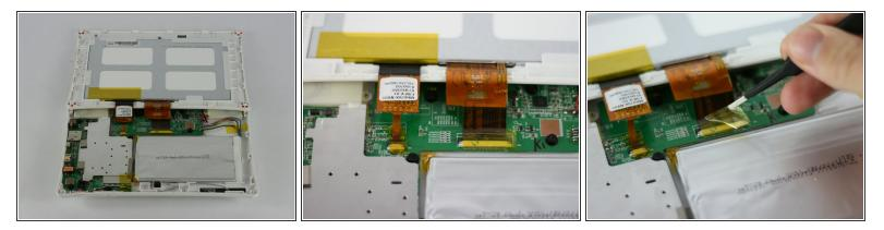
• Lay the tablet down flat and remove the yellow tape from the ZIF connector on each side
