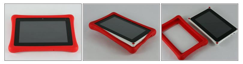
• Remove the rubber bumper from the tablet.
