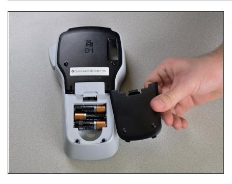
Remove the compartment cover to reveal the batteries. Remove the 6 old batteries.
