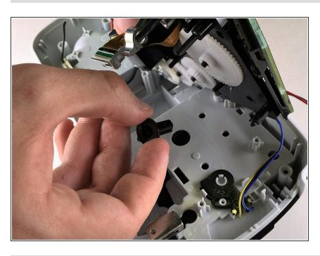
With the device components exposed, gently lift the wheelhead out of the label maker.
