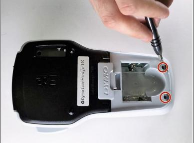
Using a Phillips #0 screwdriver, remove the four 1.3mm screws from the cartridge compartment and two 1.2mm screws from the battery compartment.
