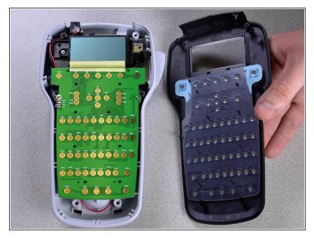
Using a spudger or other tool, lift and remove the front of the device.
