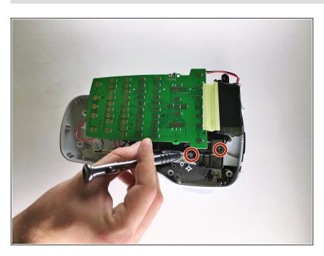
Lifting the circuit board, use a Phillips #1 screwdriver to remove the two 1.2mm screws from under the circuit board.
