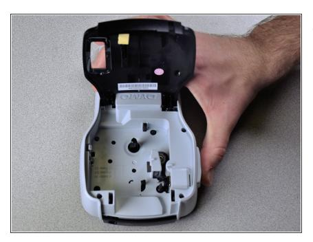
To open the cartridge compartment, simply lift on the front of the device.
