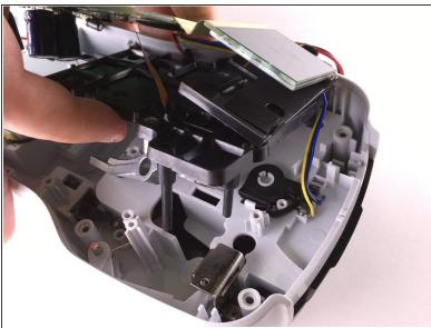
Proceed to lift the excess device components until the rollerblade is visible.
