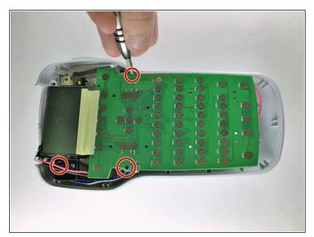
Using a Phillips #0 screwdriver, remove the three 1.1 mm screws from the circuit board.
