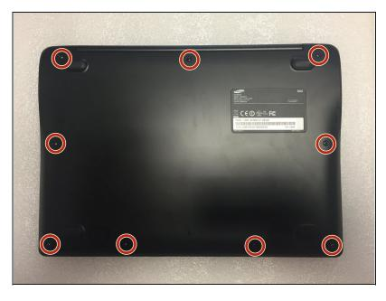
Using a PH0 bit, remove all 9 screws from the edges of the case.
