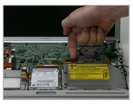
Disconnect the large black connector from the logic board and get out from under the red and black speaker cable.
