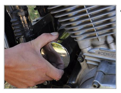
Carefully thread your new oil filter into place, turning it in a clockwise direction. Do not overtighten your filter. Only turn the filter a 1/2 turn past the point where you start to feel resistance from the gasket contacting the engine.
