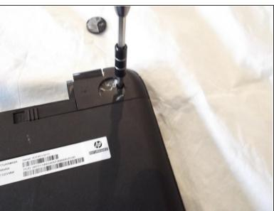
Remove the two 4mm Phillips #1 screws located under the rubber bumpers.
