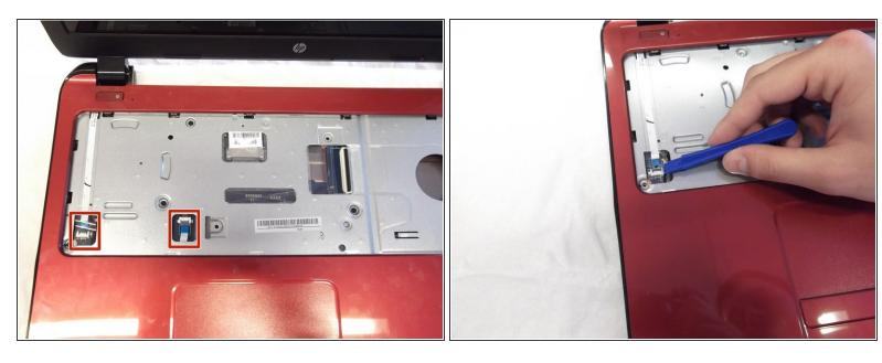
Using the plastic opening tool you will need to remove two pieces of tape.
