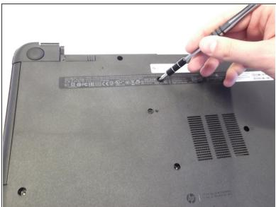
Next locate and unscrew the two 4mm Phllips #1 screws with the keyboard symbol located towards the middle and top of the bottom of the laptop.
