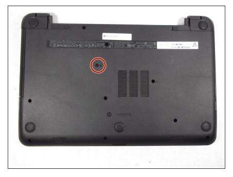
Remove the 4mm Phillips #1 screw located towards the middle of the laptop slightly towards the right with the picture of the CD next to it.
