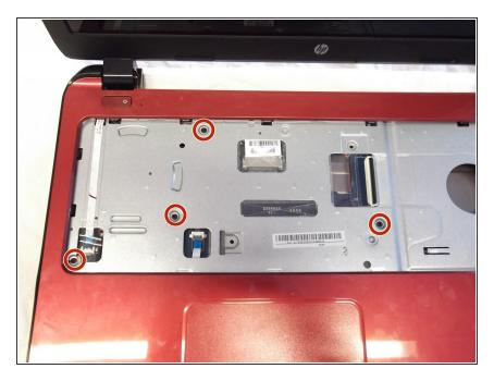
Now flip the laptop back over and open the screen. Remove the four 4mm Phllips #1 screws.
