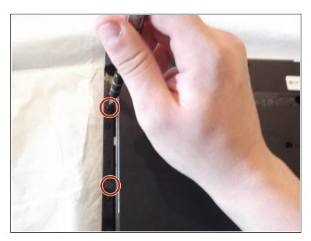
Remove the two 4mm Phillips #1 screws located where you pulled the disk tray out of.
