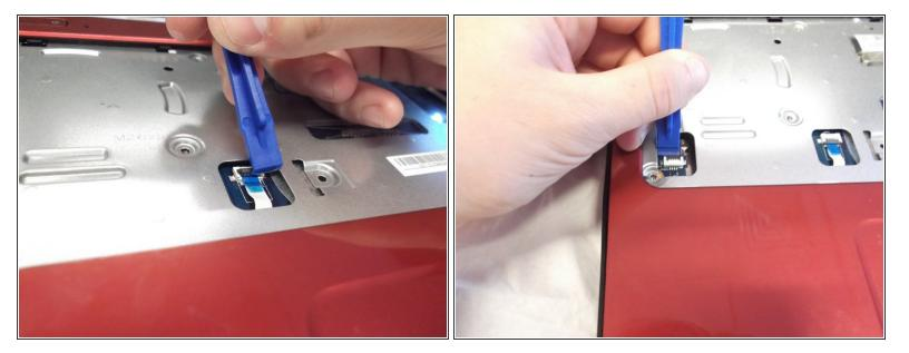
Using the plastic opening tool detach both ribbon cables by disconnecting both ZIF (zero insertion force) connectors on the ends.
