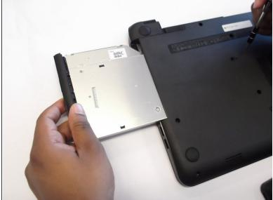
Slide the disc tray out of the its slot.
