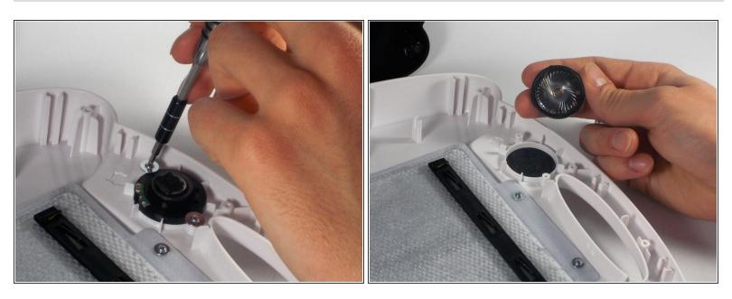
Remove the 2 5mm PH 0 Phillips screws with 10 mm heads that secure the speaker to the front of the case.
