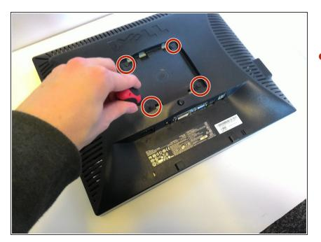
Remove the 4 black screws on the back of the monitor. This detaches the screen and housing from the case internally.
