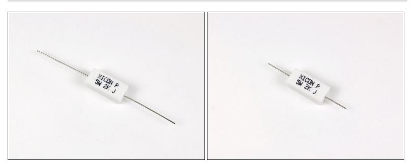
Next, trim both of the leads leaving the resistor to match the length of insulation stripped off the wires in the previous step.
