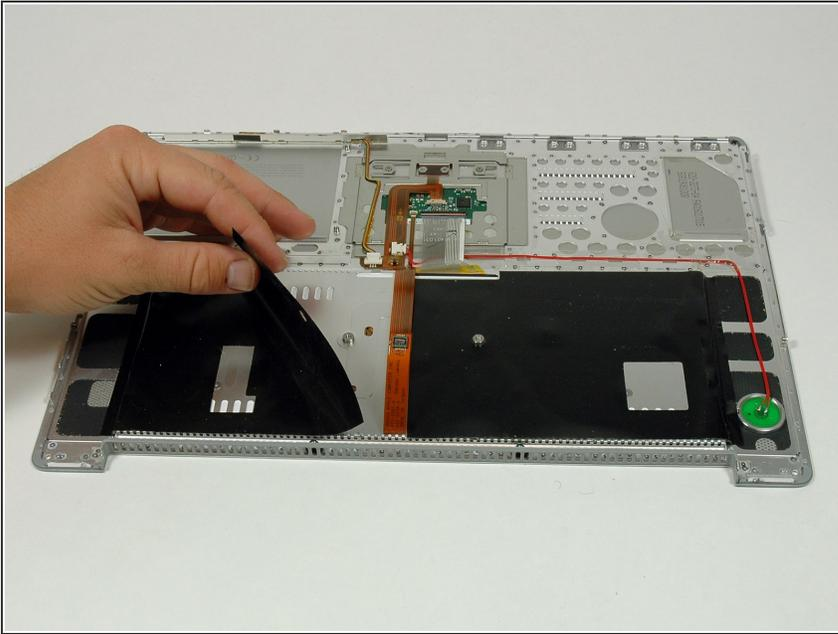
**⚠** On the following step, be careful with the tape on the side of the keyboard with the green power button, as the tape may stick and tear.
