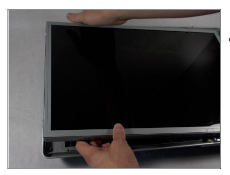
Lift the screen assembly from the plastic housing from the corners.
