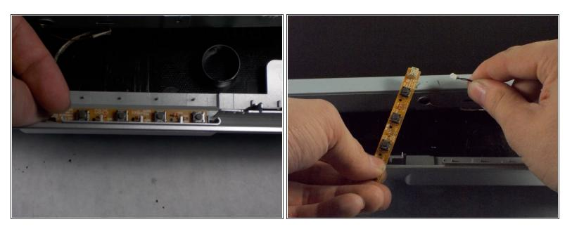
• Remove the wire connecting the contacts to the screen assembly.
