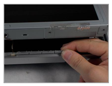
• Remove the plastic buttons from the contacts
