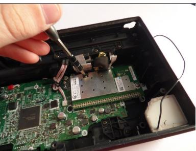
Remove the two Philips J1 10mm screws from the top side and right side of the AM/FM chip.
