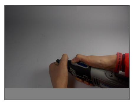
Remove the collar wrench by pushing the gear lock button.
