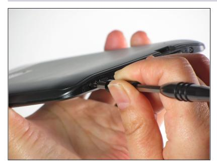
Remove two 3mm screws with the Phillips screwdriver.
