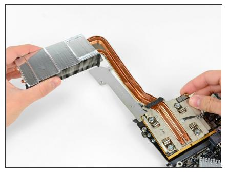
• Lift the GPU heat sink slightly and pull the GPU board out of its socket on the logic board.
