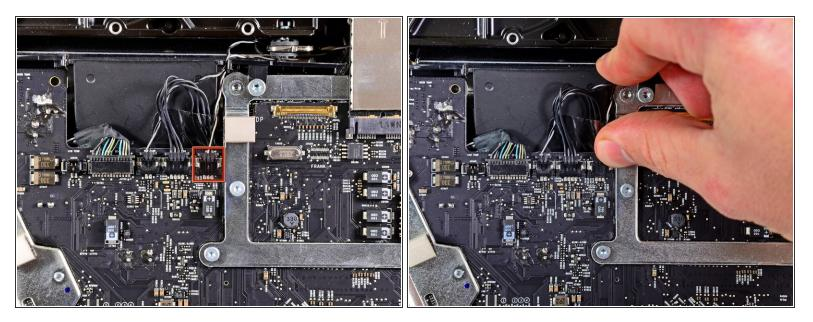
Pull the optical drive thermal sensor connector toward the top edge of the iMac to disconnect it from its socket on the logic board.
