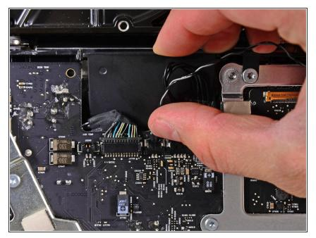
Pull the hard drive thermal sensor cable out of its socket and toward the top edge of the iMac to disconnect it from the logic board.
