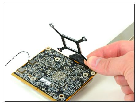
• Remove the clamping bracket from the back of the GPU.
