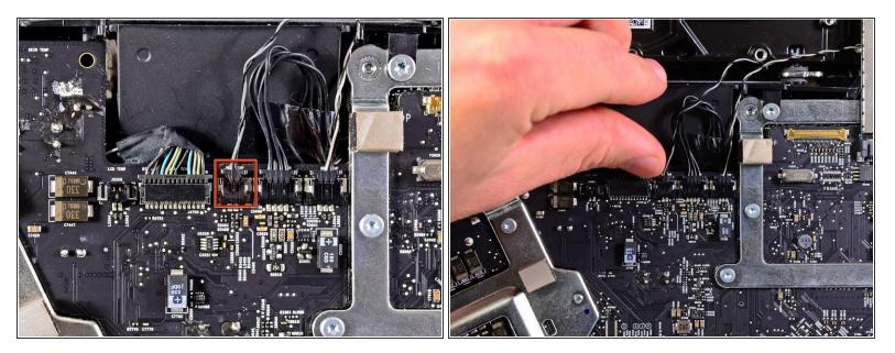
Pull the hard drive temperature sensor connector toward the top edge of the iMac to disconnect it from its socket on the logic board.
