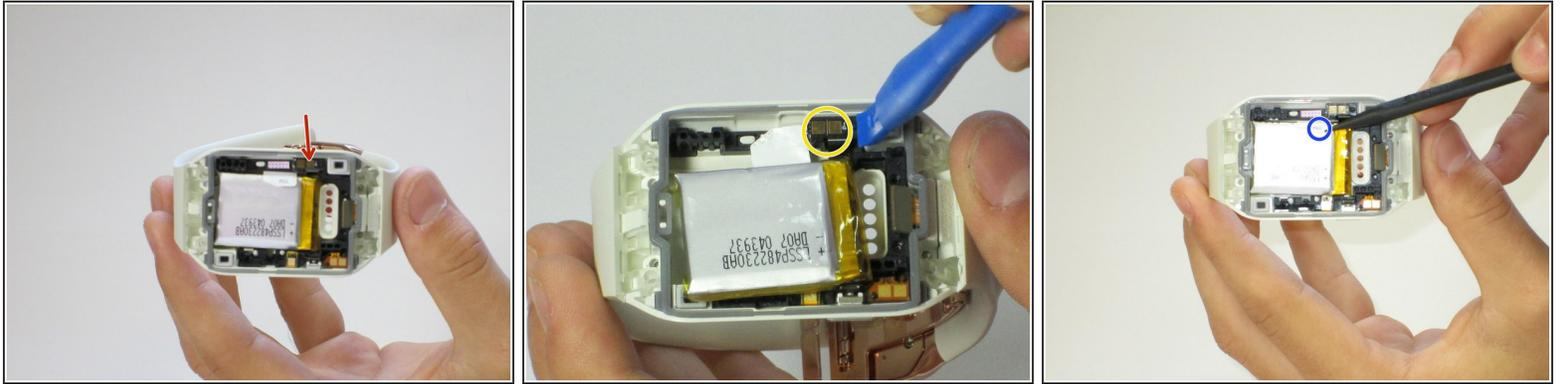
**⚠** Notice the leads attached to the base of the watch. You will need to remove this before you pull the battery out.
