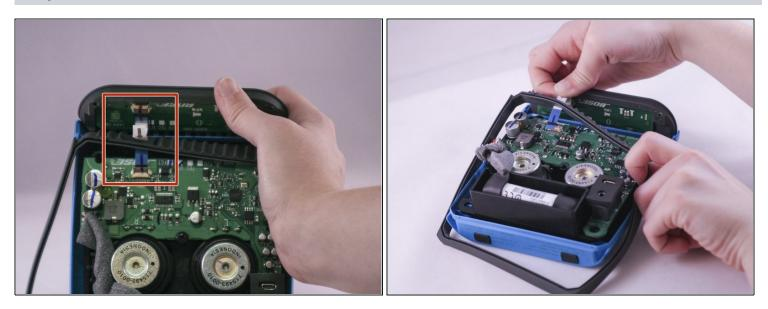
• Carefully pull the ribbon cable through the rubber gasket that runs around the device.
