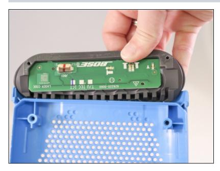
To remove the old rubber button pad, carefully peel it off of the blue casing.
