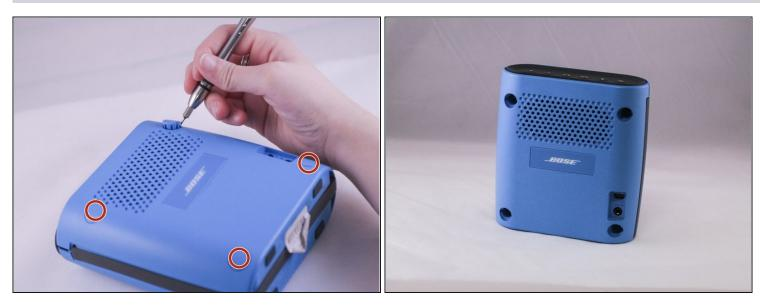
(i) Four round, plastic plugs are located on the back of the device.
