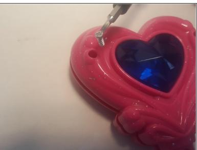
Use a Phillips #0 screwdriver to remove every screw on the back of the wand.
