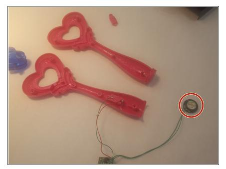
Locate the speaker at the bottom of the wand, and take it out.
