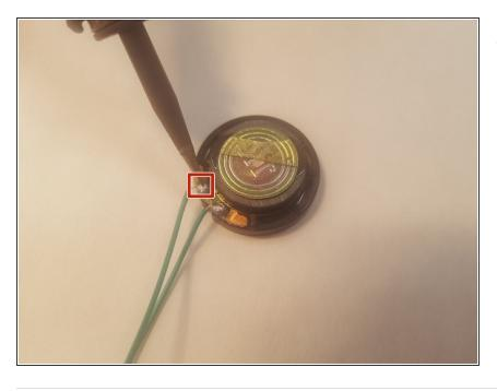
Desolder the speaker wires from the terminals on the speaker.
