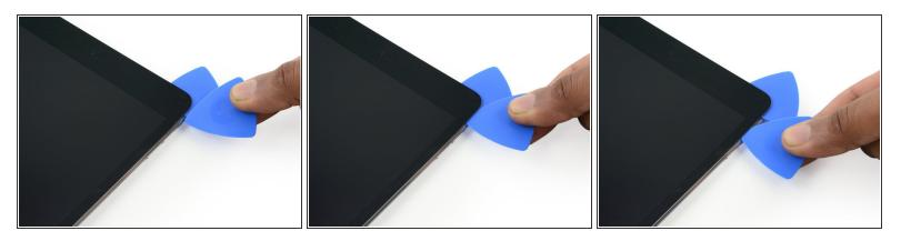
• Insert a new opening pick and slide it down the right edge of the iPad, releasing the adhesive as you go.
