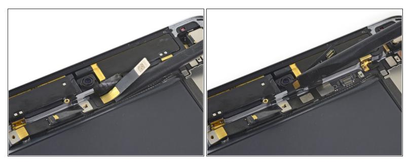
• Push back the front-facing camera's ribbon cable to access the headphone jack connector.
