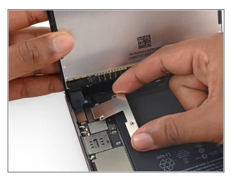
• Remove the battery/display cable bracket.
