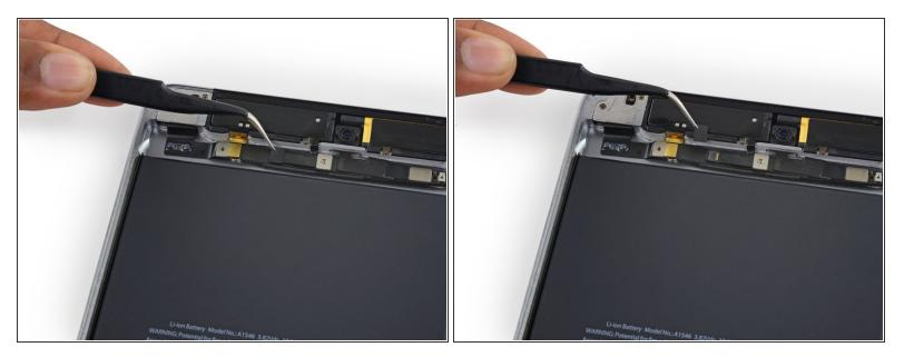
Use tweezers to remove the small piece of tape covering the the left antenna ribbon cable ZIF connector.
