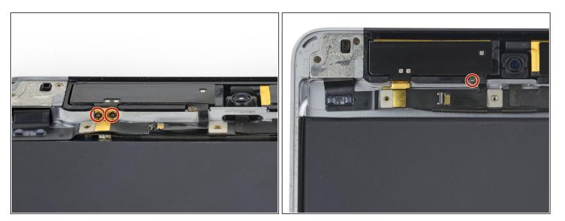
• Remove the three 1.4 mm Phillips screws securing the upper left antenna to the rear case.
