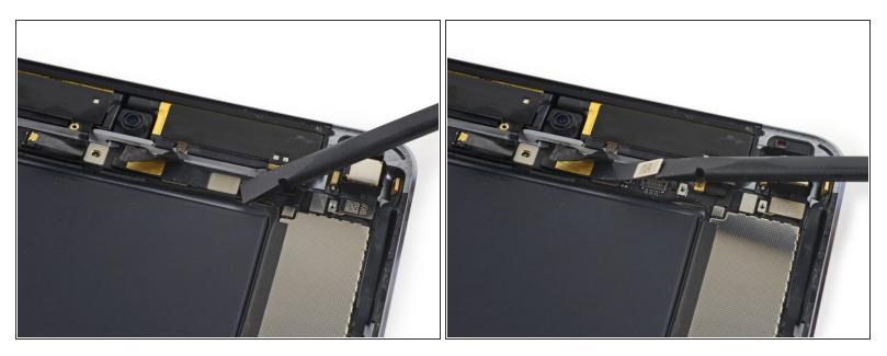
Use the flat end of a spudger to disconnect the front camera press connector from its socket on the logic board.
