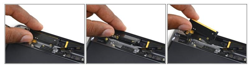
• Lift up and remove the upper left cellular antenna.
