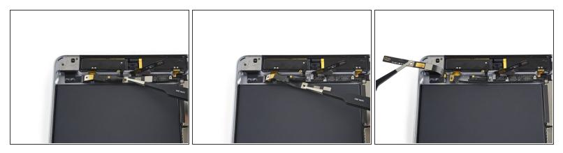
• Gently fold the headphone jack ribbon cable back to reveal the antenna interconnect cable under the left antenna.
