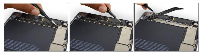
• Use tweezers to peel up the looped tape adhered over the upper component cable bracket.
