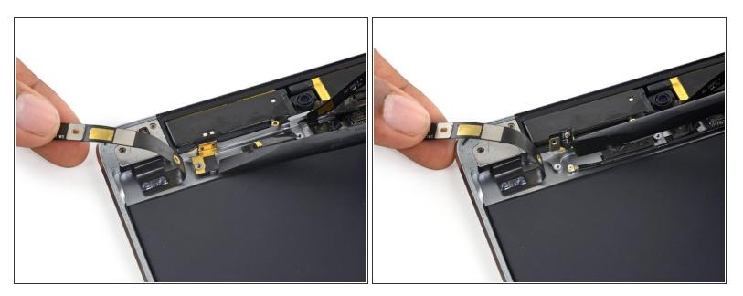
Use the flat end of a spudger to lift up the left antenna's connector and disconnect it from its interconnect cable.
