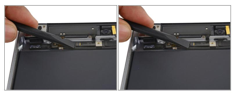
Use the flat end of a spudger to flip up the retaining flap on the left antenna ribbon cable ZIF connector.
