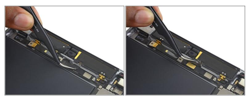
• Peel up the tape over the front camera ribbon cable.
