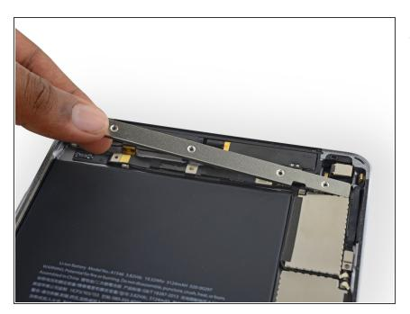
• Remove the upper component cable bracket.
