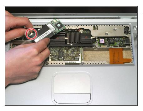
Disconnect the connector cable from the modem.
