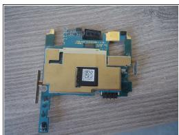
Careful, the board won't go without unscrewing this tiny screw, securing the top speaker (sorry for the quality)!
