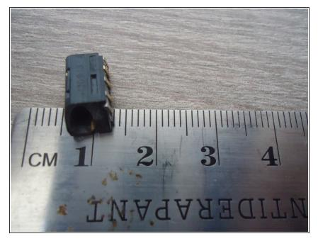
The female Jack connector is not soldered at all! Only on its place, with the four connectors touching thr motherboard.
