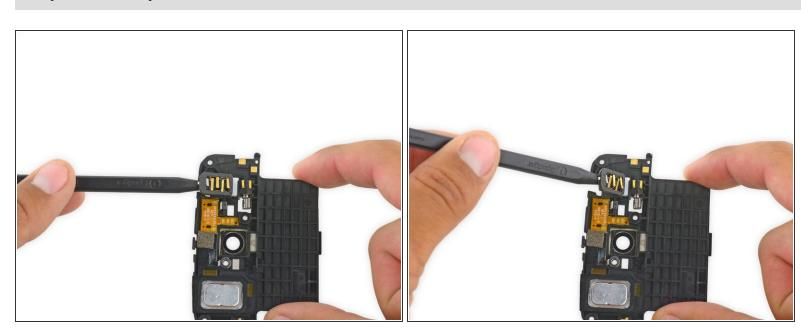
Insert the pointed end of a spudger into the headphone jack, and gently pry the jack up and away from the midframe.
