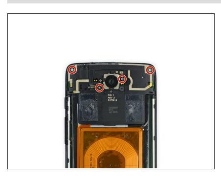
Remove the four Torx T5 screws securing the midframe plate.
