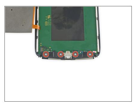
Remove the four Torx T5 screws securing the lower antenna board to the motherboard.
