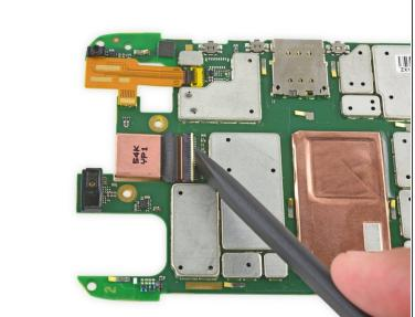
Use the flat end of a spudger to flip up the tan retaining flap on the rear-facing camera ZIF connector.
