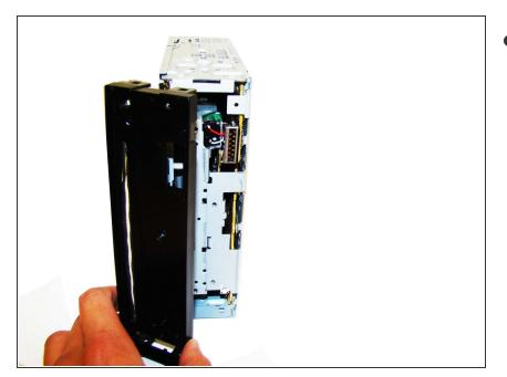
Remove the black front plate of the stereo.
