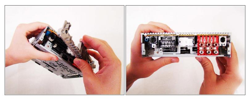
• Firmly grip the body of the stereo and pull off the silver back plate.
