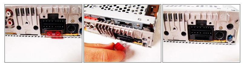
• Carefully pull the fuse out of the back of the stereo.
