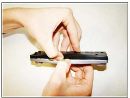
Use two fingers to create a small gap in the top of the faceplate, as indicated in the picture.
