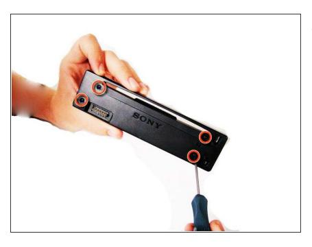
Using the <u>Phillips #0 Screwdriver</u>, unscrew the 4 (length - 11.11mm) screws on the front screen.
